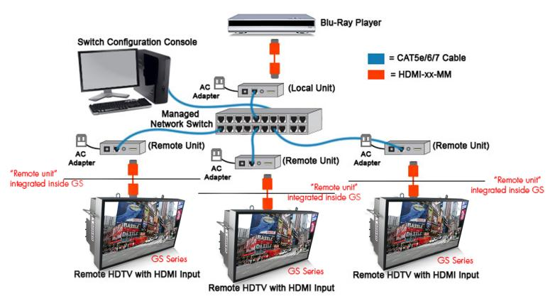
The Suntronic's GS Series with <u>CIP900-IP-TR</u> is an integrated all-in-one monitor features Video-over-IP this technology for a fully seamlessly solution that integrates easily into your existing system.
